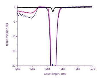
0.35nm. Mismatching LR grating relative to HR one is up to  $\pm~0.15$ nm. For fiber lasers with narrow line we are presented FBG pairs with FWHM around or less 0.1nm with ideal matching without adjustment. The transmission spectrum of FBGs Pair for Yb laser and Raman converter are presented in the graph.
